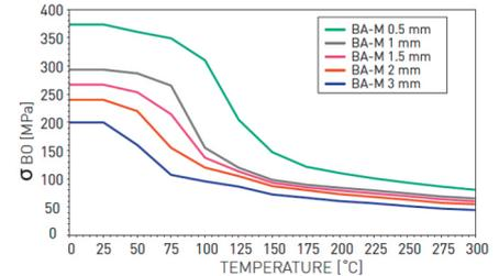
σ<sub>BO</sub> diagram represents σ<sub>BO</sub> values for different gasket material thicknesses. These values indicate the maximum in-service compressive pressures which can be applied on the gasket area involved without destructing or damaging the gasket material.
